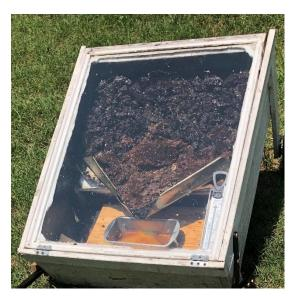
Wax can easily be processed in a solar wax melter. Nice blocks of yellow wax can be collected.
