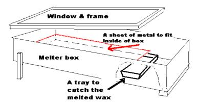
The size of the window will determine all other dimentions. The sheet metal will hold burr comb, wax from cappings, etc. The window lid must fit tight to hold in heat from the sun.
