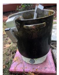
Slum-gum from the solar wax melter can be placed in a cloth bag which is then placed in a turkey cooker. An electric heater makes it easier to control the temperature of the water.
